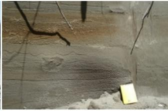
The soils in the area were weakened by lenses of fine sand that erode easily.
